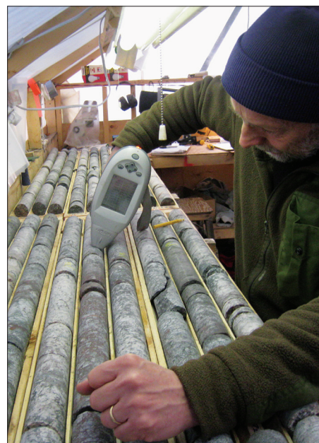
Senior Geologist Chris Pedersen analyzes rare earth contents in the rocks using a Niton XRF analyzer.
