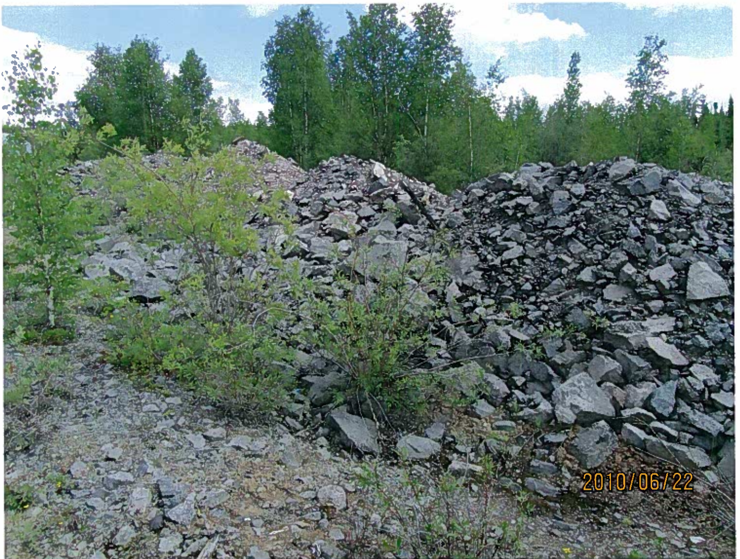
MV2010G0001 - Avalon Rare Metals Inc. - Thor Lake Piled rock at the T-zone from the decline development that will be used during airstrip construction.
