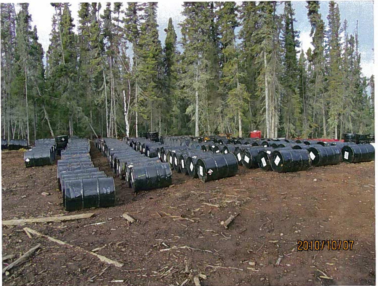
Photo #11 - Fuel cache on the south side of Thor Lake. The Inspector appreciates the Permittee's diligence with maintaining walkways between the drums for ease of inspection, and placing the bungs at 3 and 9 o'clock.
