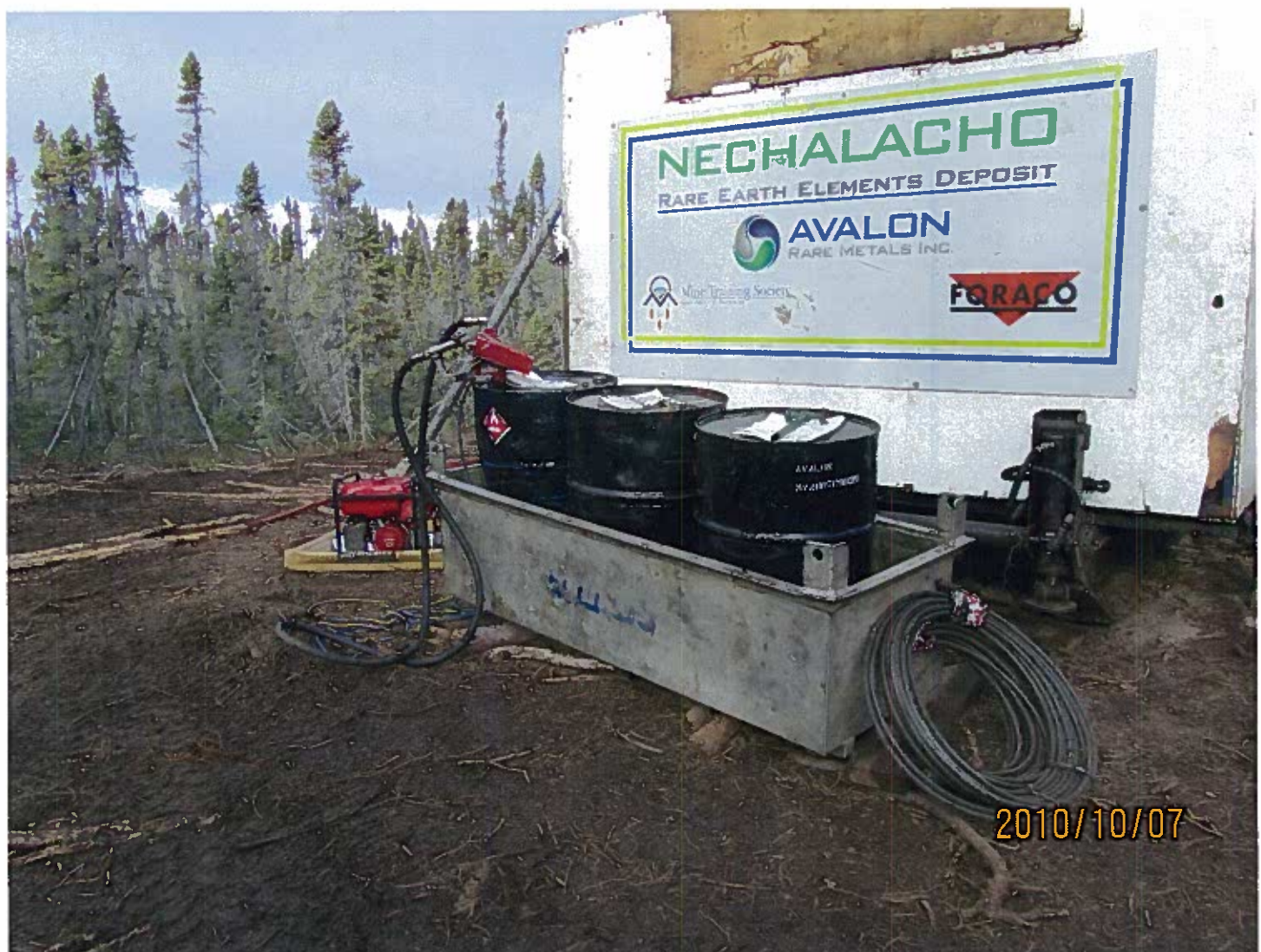
Photo #2 - Adequate secondary containment has been implemented on active drums at the skid mounted drill.
