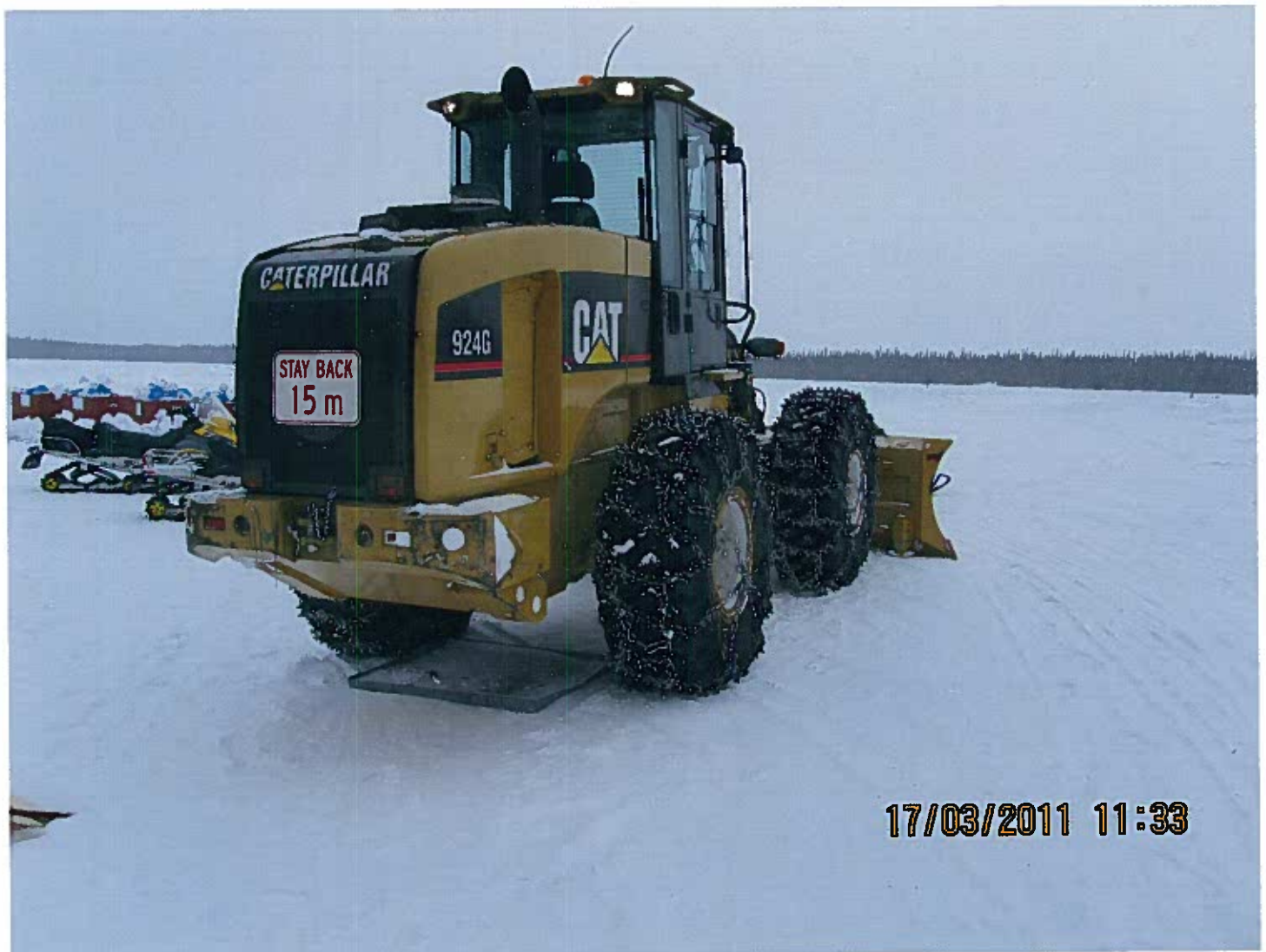
MV2007C0039 - Avalon Rare Metals Inc. - Mineral Exploration - Thor Lake, NT. Drip trays have been placed under equipment on site.
