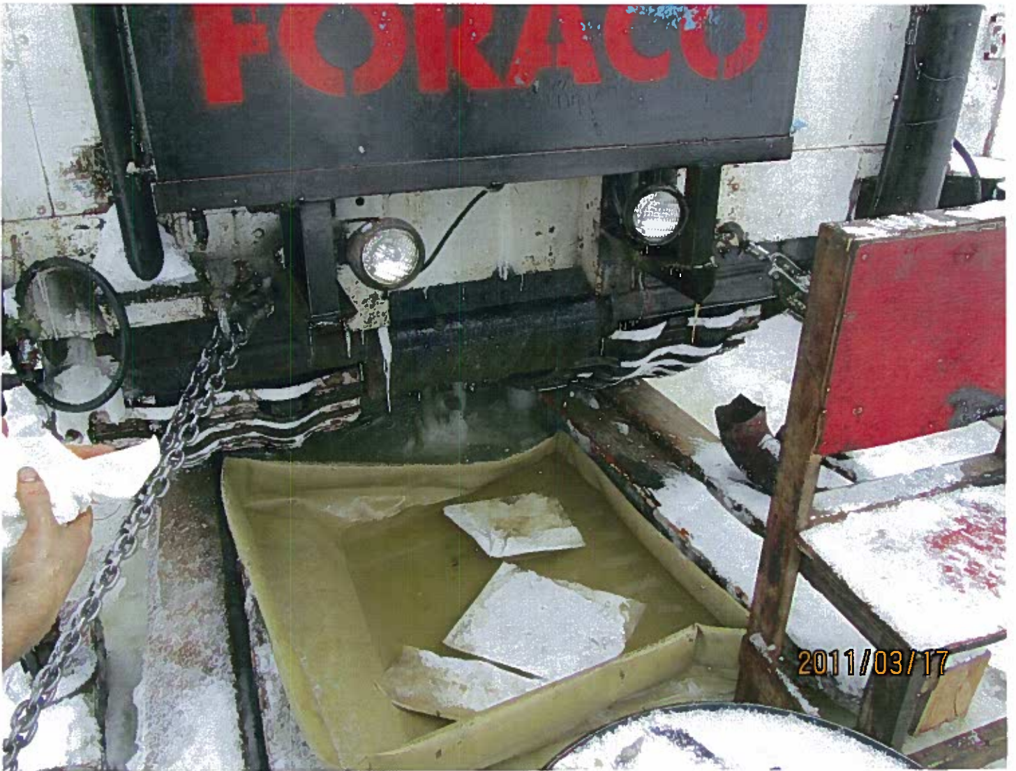
MV2007C0039 - Avalon Rare Metals Inc. - Mineral Exploration - Thor Lake, NT. Diesel contamination under the saddle tank on the buggy drill. Secondary containment was present but some impacted ice was identified.
